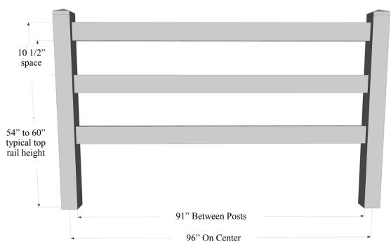
REQUIRED MATERIALS PER 8' SECTION RAILS: (3) 1 1/2" X 5 1/2" X 8' RIBBED
