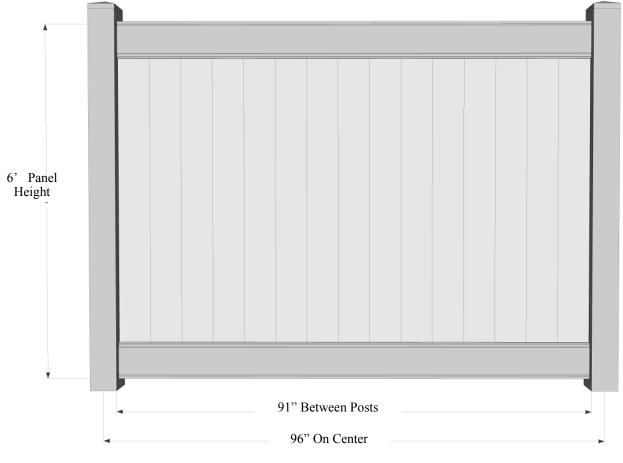
Required Materials Per 96" SectionRecommended ToolsRails<br/>2" x 7" x 94" Slotted- Measuring Tape- LevelPlanks<br/>(15) 7/8" x 6" (T&G) x 61"<br/>(2) 7/8" x 57 1/4" U-Channel- Saw- Shovel
