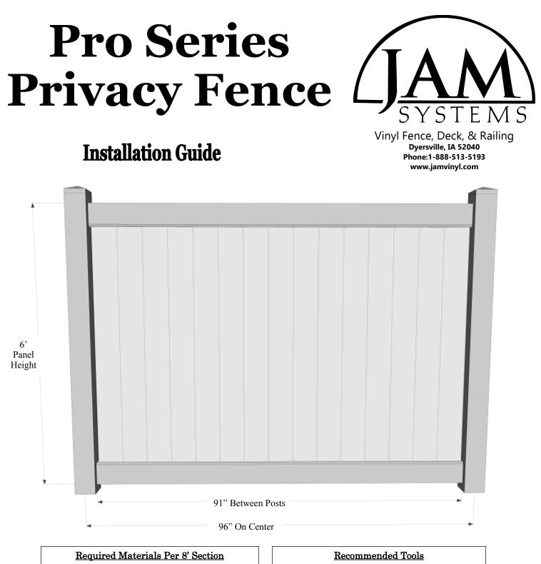
Rails 1 3/4" x 5 1/2" x 94" Slotted top rail (1) 1 3/4" x 5 1/2" x 94" Slotted bottom rail with metal reinforcing
