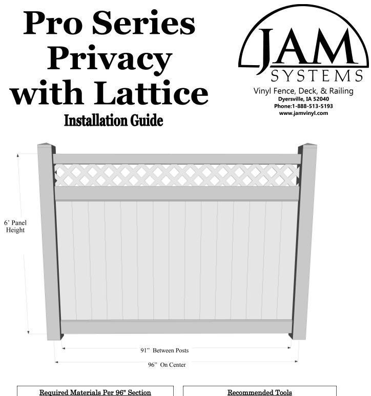
Required Materials Per 96" Section Rails (1) 1 3/4 x 5 1/2" x 94" Slotted (1)1 3/4" x 5 1/2"" x 94" Slotted & Ripped for Lattice (1) 2" x 3 1/2" x 94" Ripped for Lattice Planks (15) 7/8" x 6" (T&G) x 50 7/8"" (2) 7/8" x 47 3/8" U-Channel (1) 12" x 91" Lattice
