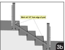
**Cutting Rails (Step Sections):**
